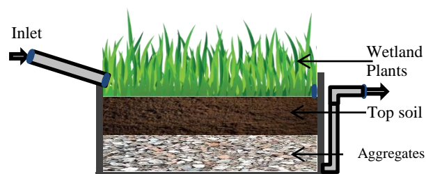
Figure 1: Experimental wetland unit
