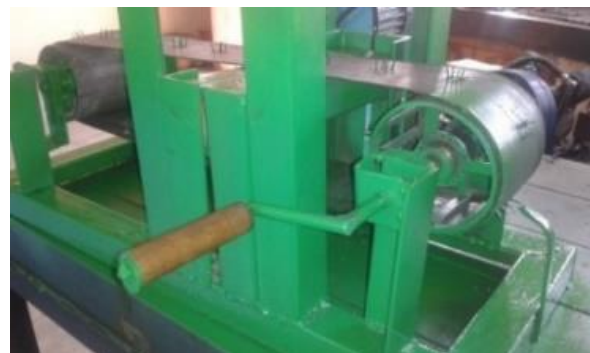
d. Operating handle of the conveyor
