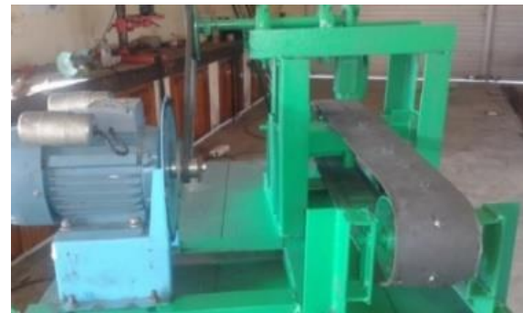
b. Electric motor, belt conveyor and hammer of the machine
