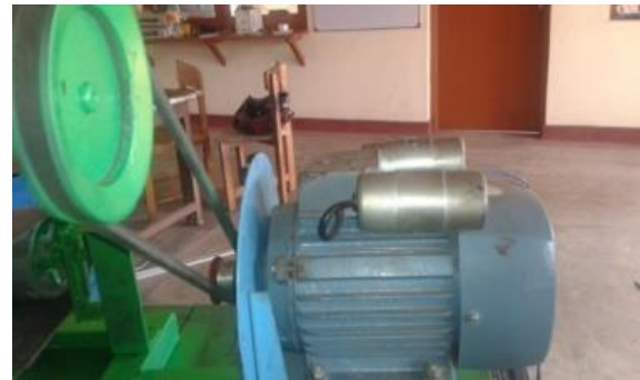
c. Power transmission from motor to hammer
